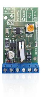
**SS14** is a vibration/inertial detector designed for the protection of windows, cabinets, fixtures, and so on. It has a high-precision vibration sensor, which allows to determine the type of shock and/or vibration caused by an attempt to break through or forcing a frame. It is not necessary to use pulse analysis boards since everything is processed within the sensor itself. It is equipped with 2 channels, contact REED and INERTIAL / FLIP.
